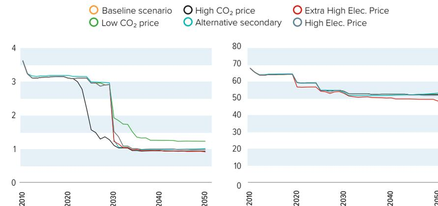
Figure 43: 2050 scenario's for aluminium production. (left) direct CO<sub>2</sub> emissions t CO<sub>2</sub>/t cast aluminium, (right) energy use GJ/t primary aluminium (Source: JRC, 2015<sup>253</sup>)
