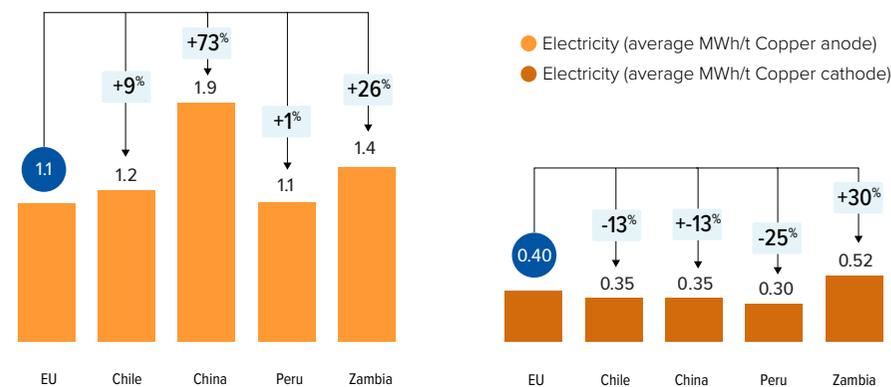
Figure 41: (left) Electricity use per tonne copper anode (MWh/t) (2013) (right) electricity use per tonne copper cathode (MWh/t) (2013) (Source:JRC, 2016)<sup>246</sup>
