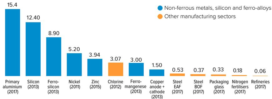
Figure 36: Average electricity use per tonne metal (MWh/t)<sup>242</sup>
