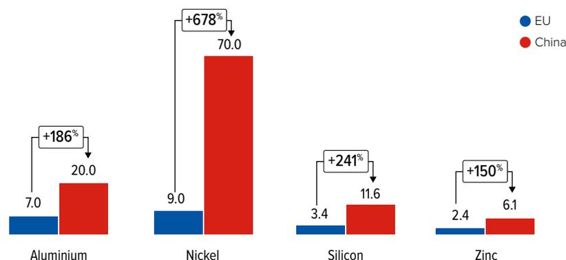
Figure 42: CO<sub>2</sub> intensity of metals production - EU vs. China (t CO<sub>2</sub>/t metal)<sup>248</sup>
